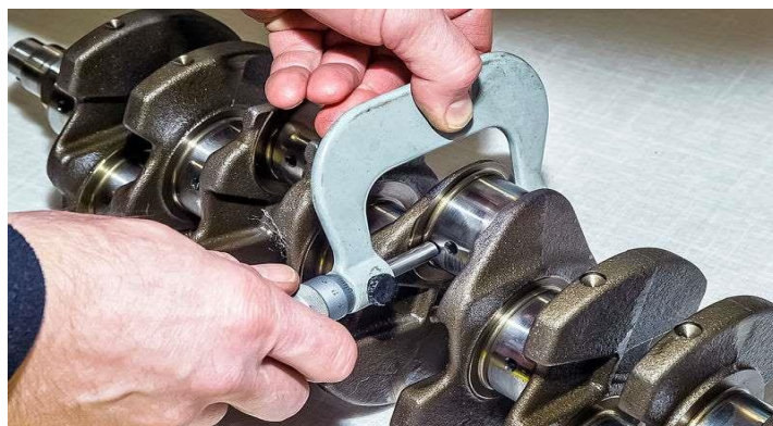
14-rasm. Mikrometr MK 50-1 bilan detalni o'lchash.
