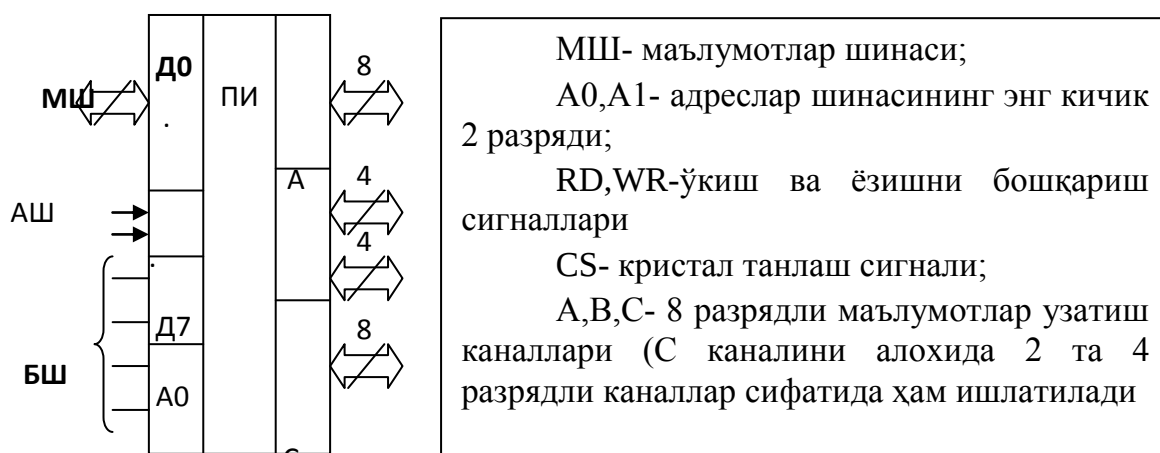
1-rasm. K580VV55 mikrosxemasining kirish/chiqish signallari.
