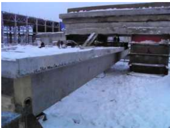
Tavr shaklli temirbeton to'sinining statik sinovi
