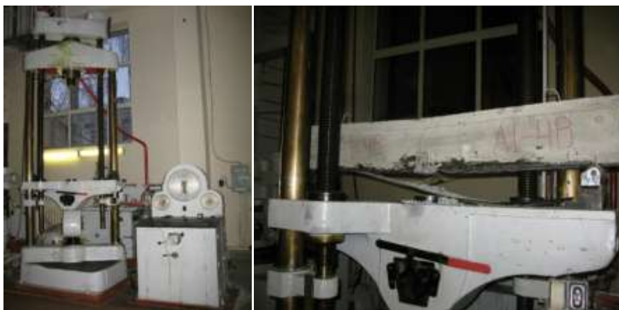
Temirbeton namunasining chidamlilikka sinovi
