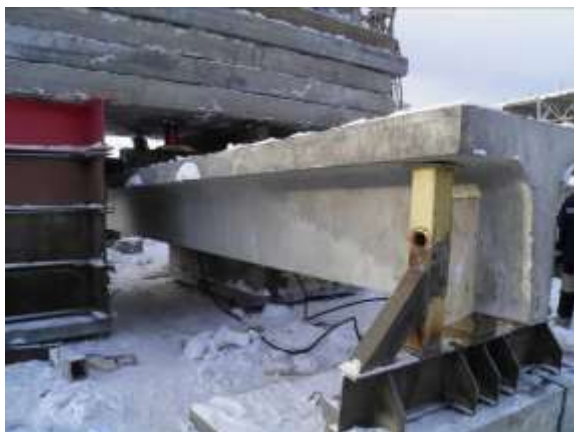
Tavr shaklli temirbeton to'sinining statik sinovi
