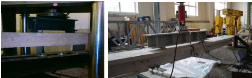
Temirbeton to'sin namunasining mustahkamlikka statik sinovi
