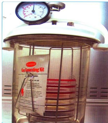
Fig. 2.3. Anaerobic jar with anaerobic cultures, Petri dishes and a bag with substances creating conditions for anaerobic and robiosis are visible
