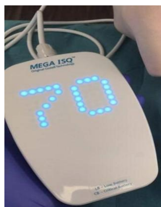
6-rasm. “Mega ISQ” (Original Osstell Technology, Shvesiya) rezonans-chastotali tahlil apparati.
