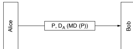
Figure 8-23. Digital signatures using message digests.
