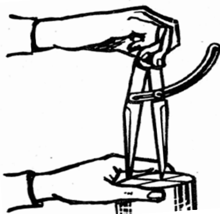
54 – rasm Rejalash sirkuli 1 – oyoqcha, 2 – sharnir, 3 – yoy, 4 – qotiruvchi vint.
