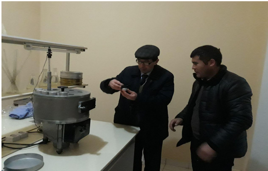
2.4.1-rasm. Laboratoriya sharoitida mahsulot namligini aniqlash.
