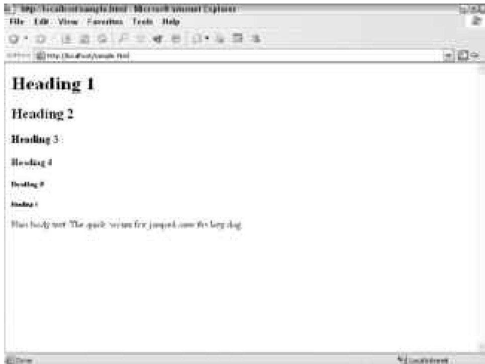
Figure 2-4: HTML supports six levels of headings.
