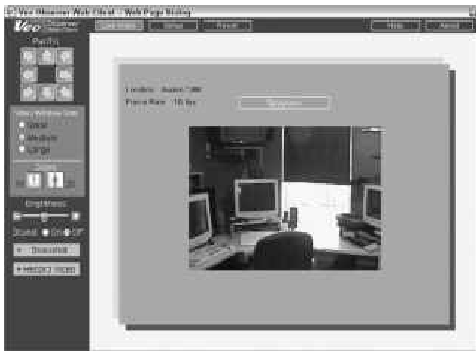
Figure 28-2: The ActiveX control used by a popular network camera to allow control of the camera over the Internet.
