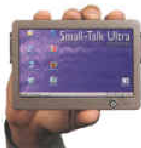
Small-Talk Ultra: a mobile computer from Galileo, which includes Windows-Lite – a screen reader for the blind.
