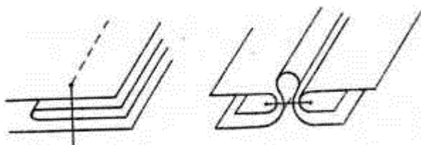
116-rasm. Mag‘iz chokli baxyaqator.
