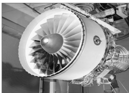
7-rasm. Metall qotishmadan yasalgan turbo dvigatel suratii.
