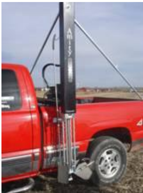
10.7.3.2-rasm. Avtomobil kabinasi ichidagi yoki kuzoviga maxkamlangan sinov namuna olish qurilmasi
