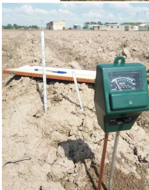
5- rasm. Soyani ekishdan oldingi dala sharoitida tuproqning pH darajasi(A) va haroratini(B) o‘lchash jarayoni
