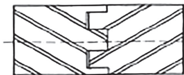
19.2-rasm. Tishlarining yo'nalishi turlicha bo'lgan yig'ma freza
